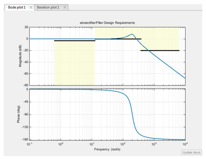
The **Bode plot 1** window in the **Response Optimizer** shows that the model output goes out of the region bounded by the design requirement line segments.
