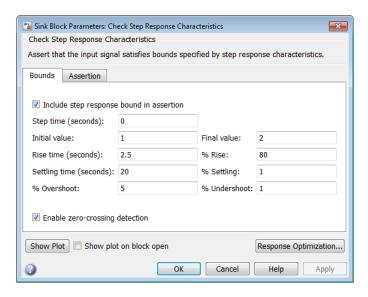
Instead of specifying time-domain requirements in the Check blocks, you can specify them in the **Response Optimizer** without adding blocks. For an example that uses this approach, see "Design Optimization to Track Reference Signal (GUI)" on page 3-19.
